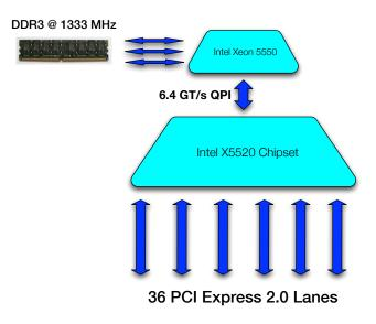
Fig. 1. Typical architecture of an Intel Xeon 5550 and 5520 chipset.
