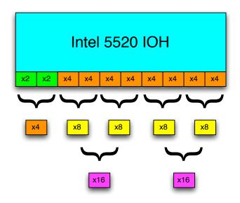
Fig. 7. Intel 5520 chipset PCI Express combinations
