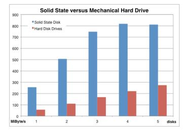
Fig. 2. Disk array read performance for up to five solid state disks.
