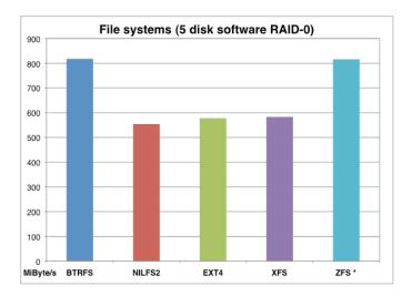
Fig. 5. Read performance with different file systems. ZFS runs under FreeBSD, the other file systems under Ubuntu Linux.
